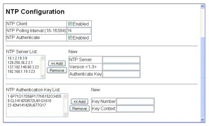
Figure 3-22 NTP Client Configuration
