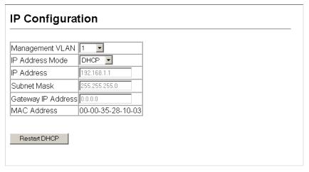
Figure 3-7 DHCP IP Configuration
