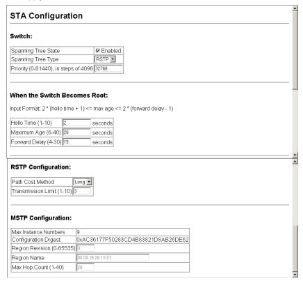
Figure 3-85 Configuring Spanning Tree
