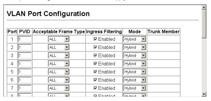
Figure 3-97 Configuring VLANs per Port
