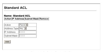
Figure 3-64 Configuring Standard IP ACLs
