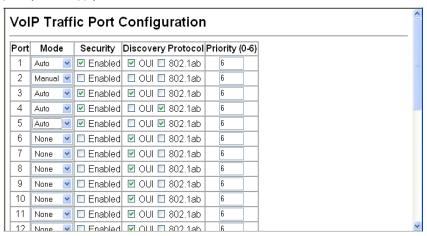
Figure 3-125 VolP Traffic Port Configuration
