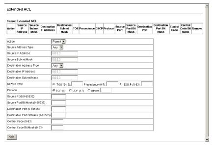
Figure 3-65 Configuring Extended IP ACLs
